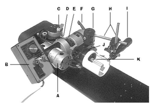
For those not acquainted with the O.M.F., it is a machine that cuts \*curved\* facets, which can add extra brightness and scintillation to gem designs. That means the design possibilities of gemstones are virtually limitless with this O.M.F. Machine. This machine is used to apply concave facets to gemstones to improve the optical effects. The instrument consists of a grind/polish assembly to which the facet gem from your standard faceting machine is attached.
